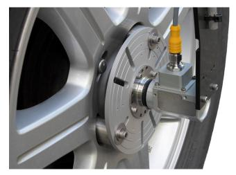
An adapter plate enables an assembly to mount to a variety of bolt circle patterns. Michigan Scientific offers many standard wheel adapter plates, used for mounting instrumentation to a wheel. Wheel adapter plates can also be customized for a specific application.
